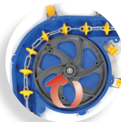
Pulleys that prevent feed from gathering.
